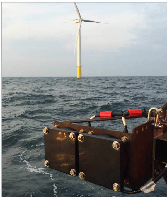
Example of transducers used with EBP system to detect export and infield cables.
