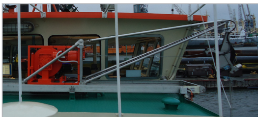
Winch used to enable RheoTune measurements.
