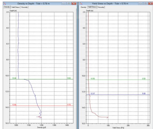
RheoTune software displaying both density (left) and yield stress (right).
